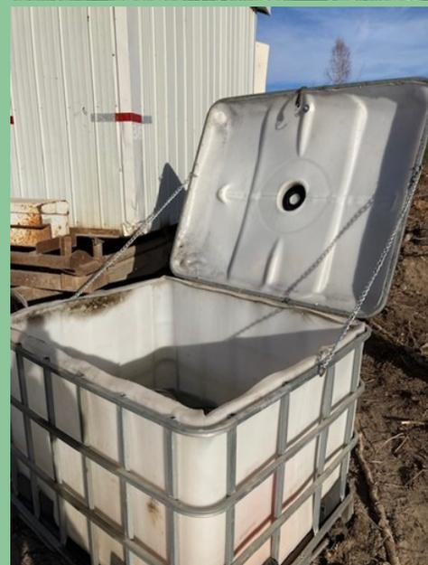
These photos show the plastic tote modified by a Mistik contractor for storage and shipment of waste oil buckets and jugs. Typically the empty containers are stored and transported individually. This method reduces the likelihood of drip-page and leaks.
